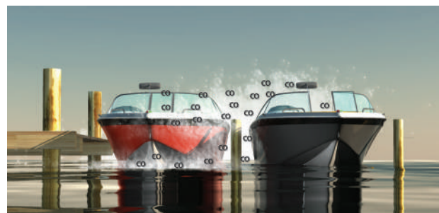
Exhausts from other vessels in confined areas.
