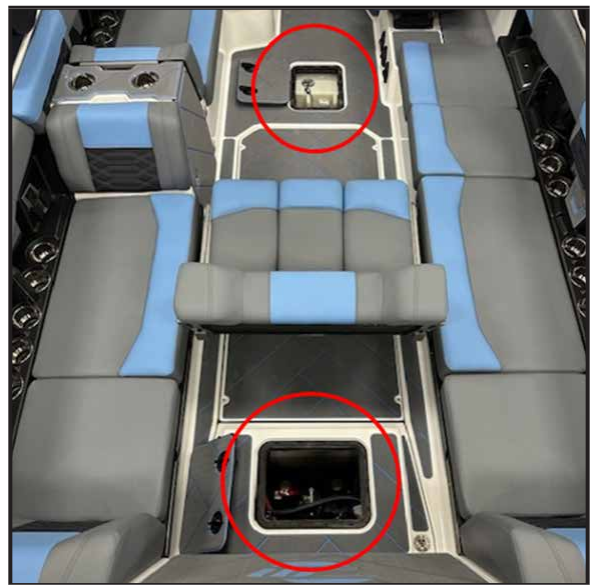
Fill pump valves and bilge T-handles are accessible through the fore and aft access panels (shown above, circled in red).
