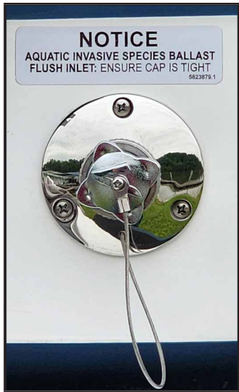
Ballast tank flush kit port, located on starboard side of the transom.
