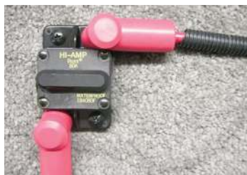
Figure 4-7. Main Circuit Breaker
