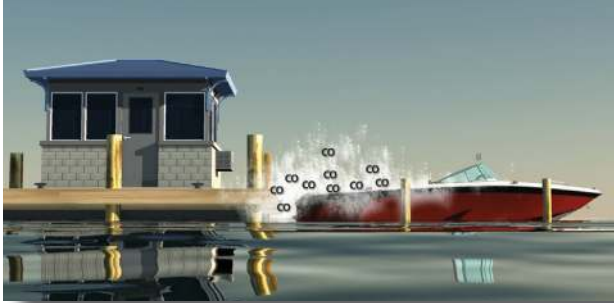
Blockage of boat exhaust by obstruction.
