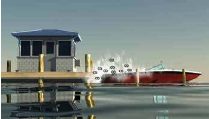
Blockage of boat exhaust by obstruction.
