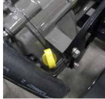
Transmission dipstick (red); V-Drive dipstick (yellow).
