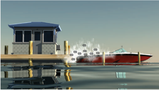
Blockage of boat exhaust by obstruction.
