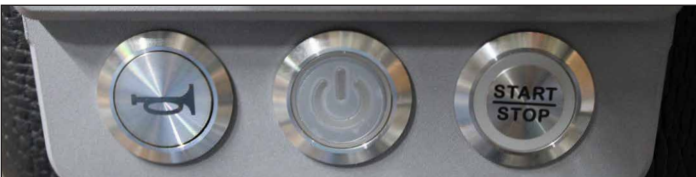
Dash buttons (from left to right): horn, power, START/STOP.
